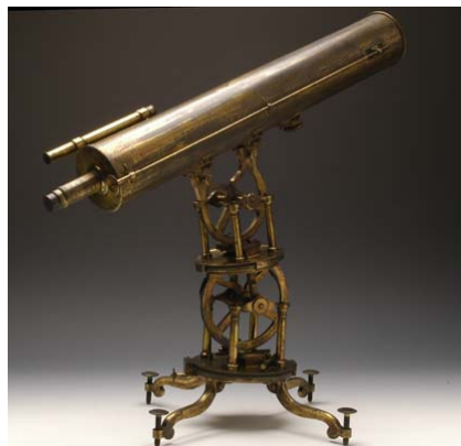
Fig.3.5: Gregorian reflecting telescope with equatorial mounting; ray diagram for the telescope
